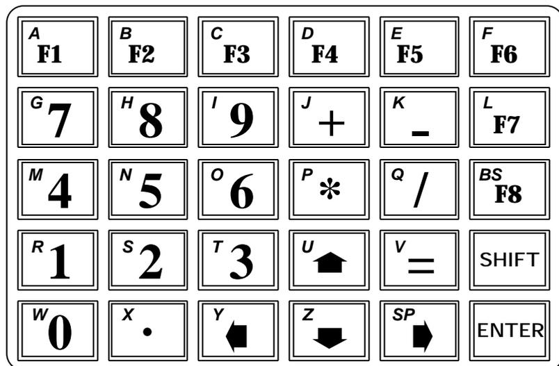
There are three keyboard modes - Upper case characters (U), Lower case characters (L) and Numeric/Command (N). The current keyboard mode, U, L or N, is shown in the bottom right corner of the LCD.
