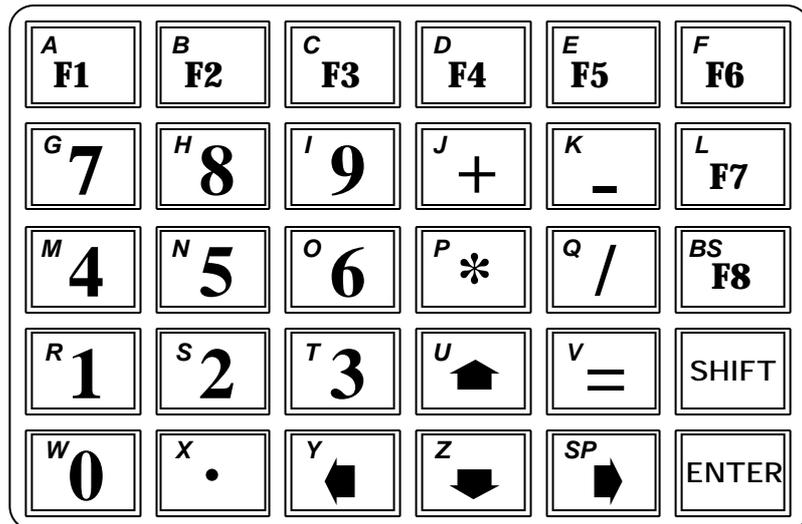
There are three keyboard modes - Upper case characters (U), Lower case characters (L) and Numeric/Command (N). The current keyboard mode, U, L or N, is shown in the bottom right corner of the LCD.
